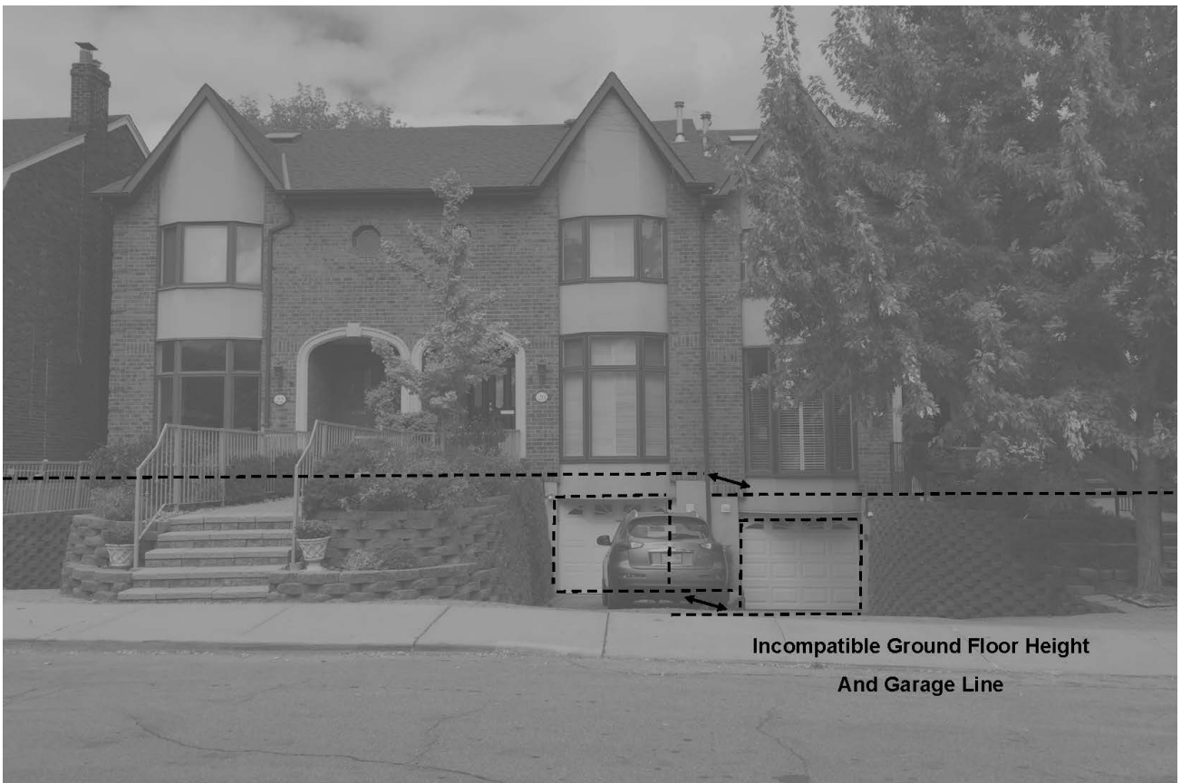
Figure 2.3f: Incompatible Ground Floor Height and Garage
