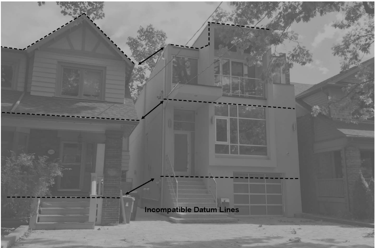
Figure 2.3e: Incompatible Ground Floor Height and Datum Lines
