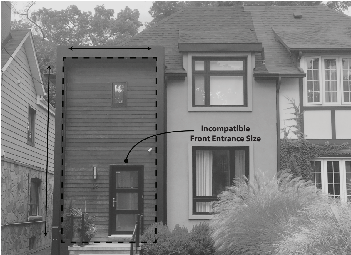
Figure 2.4c: Incompatible Scale of Front Entrance Design
