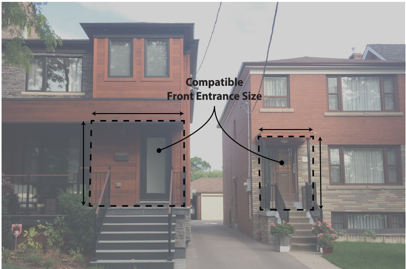
Figure 2.4d: Compatible Scale of Front Entrance Design
