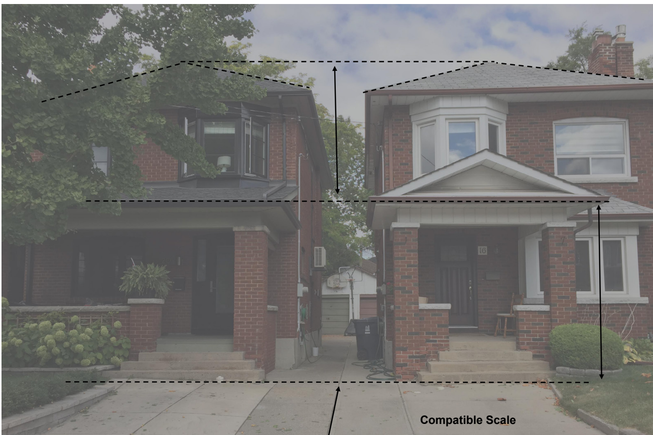
Figure 2.3b: Compatible Datum Lines and Scale
